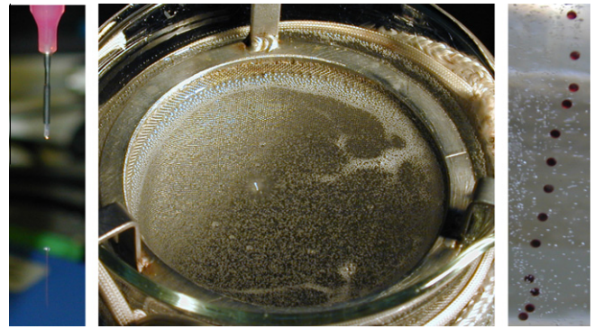
Fig. 4. Drop free fall into oil Drop free fall and bubbly oil. Left and center: Drop of zirconium solution falling into heated bath of silicone oil; bubbles were formed as the drops sank to the bottom. Right: Drops of ferric solution falling into heated silicone oil; fewer bubbles are generated.
